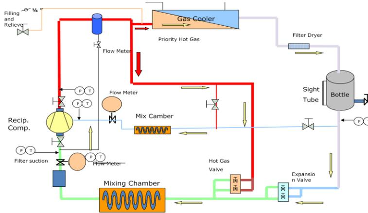
**Figure 8:** Test Rig for CO<sub>2</sub> parallel compression
