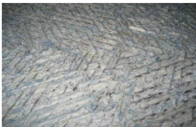
*Limescale can block your heat exchanger.*
