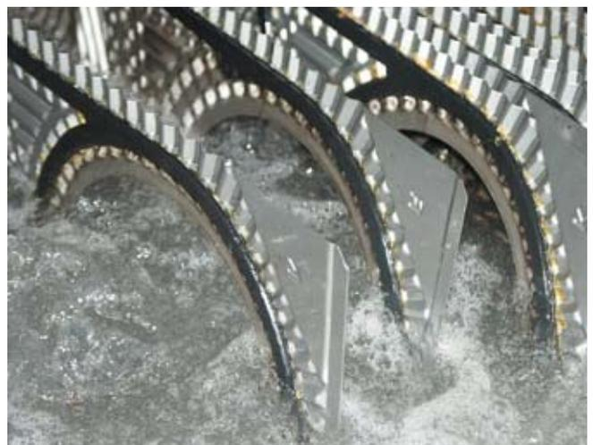
*A combination of heating and turbulence (enabled by airbubbles) results in more efficient cleaning.*
